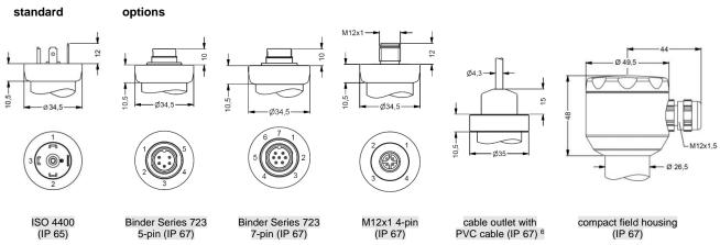
⇒ universal field housing in stainless steel 1.4404 (316 L) with cable gland M20x1.5 (ordering code 880) and other versions on request
