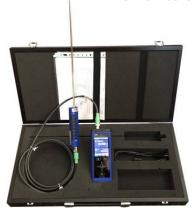
The high accurate handheld device LR-Cal LRT 1000 is used as reference standard for temperature calibration purposes. Excellent stability through multiple annealing cycles. Sensor characteristic curve is determined individually and is saved in the device. Integrated root 2 function for determination of the sensor self-heating, plus automatic elimination of parasitic thermovoltage. For traceability to national standards a DAkkS certificate of calibration is included in standard delivery.
