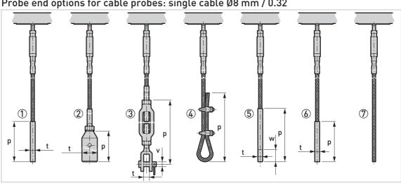
Probe end options for cable probes: single cable Ø8 mm / 0.32"
