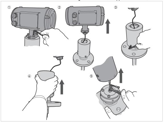
Procedure 2B: How to remove the VF04 signal converter (Ex-approved devices)
