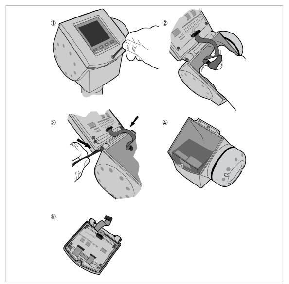
Figure 7-1: Removal of the device display cover
