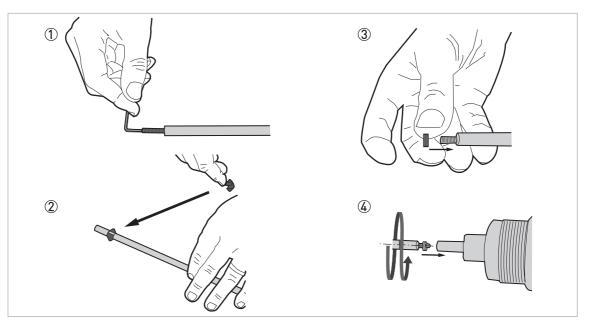
Figure 3-34: How to assemble the segmented coaxial probe: part 1
