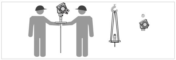
Figure 3-2: How to hold the device
