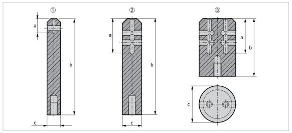
Figure 6-12: Dimensions of the counterweights
