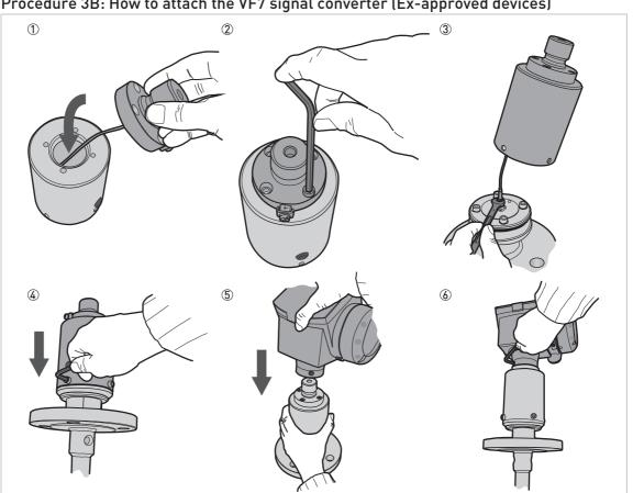
Procedure 3B: How to attach the VF7 signal converter (Ex-approved devices)
