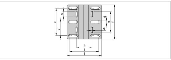
Figure 3-43: Dimensions of the wall bracket
