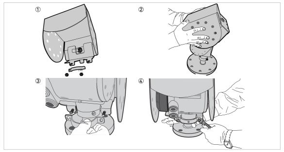
Figure 3-45: Installation of the weather protection
