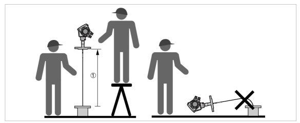
Figure 3-39: Installation of devices with cable probes (1) >1 m / 31/2 ft
