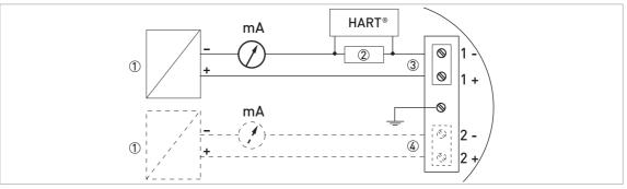
Figure 4-2: Electrical connections for non-Ex devices
