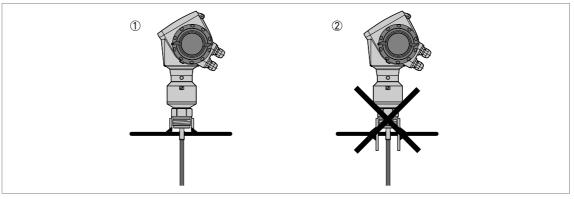
Figure 3-6: Sockets for threaded process connections
