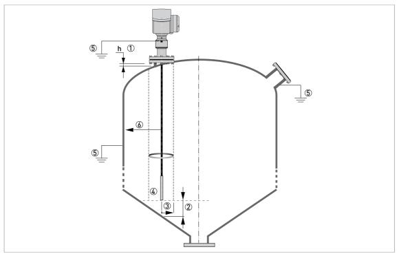
Figure 3-25: Installation recommendations for solids
