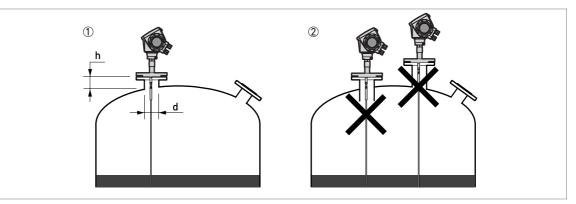
Figure 3-5: Recommended nozzle dimensions for single rod and single cable probes
