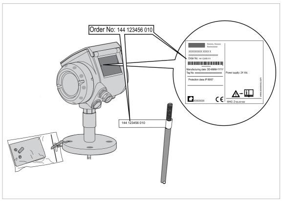
Figure 3-27: Check the order number on each component
