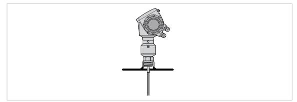
Figure 3-37: Threaded connection
