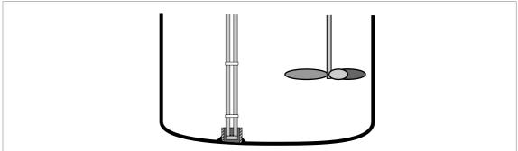
Figure 3-11: How to attach a double rod probe to keep it straight
