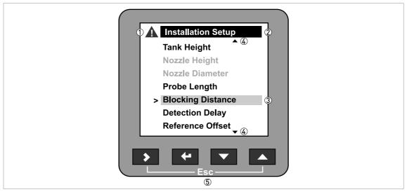
Figure 5-1: Local display screen layout
