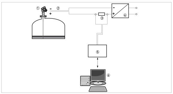
Figure 4-4: Point-to-point connection (non-Ex)
