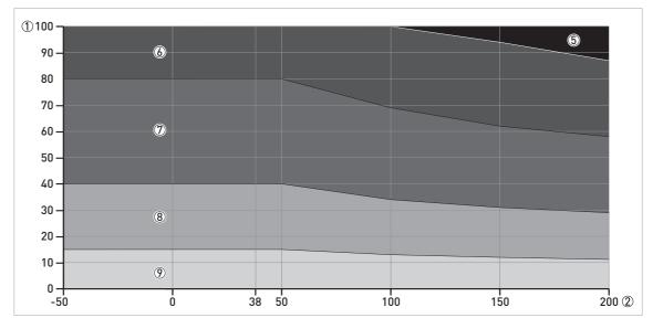
Figure 8-11: Pressure / temperature de-rating (ASME B16.5), all other probe types, in °C and barg
