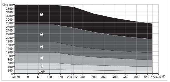
Figure 8-10: Pressure / temperature de-rating (ASME B16.5), Ø0.08<sup>°°</sup> single cable probe (HT and HT/HP versions), in °F and psig
