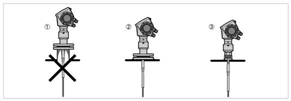
Figure 3-8: How to prevent build-up of product around the process connection
