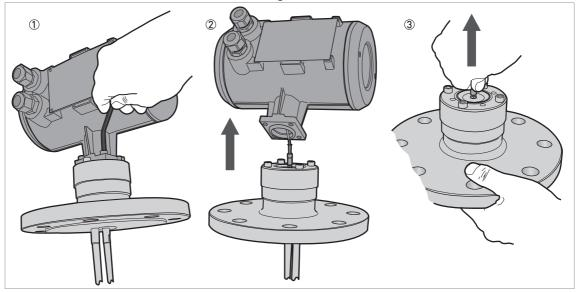
Figure 7-4: Procedure 2A: How to remove the VF04 signal converter (non-Ex devices)
