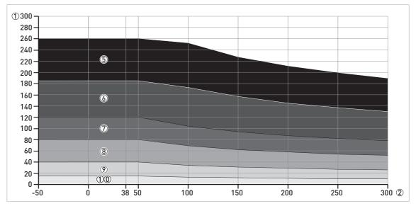
Figure 8-9: Pressure / temperature de-rating (ASME B16.5),  $\emptyset$ 2 mm single cable probe (HT and HT/HP versions), in °C and barg
