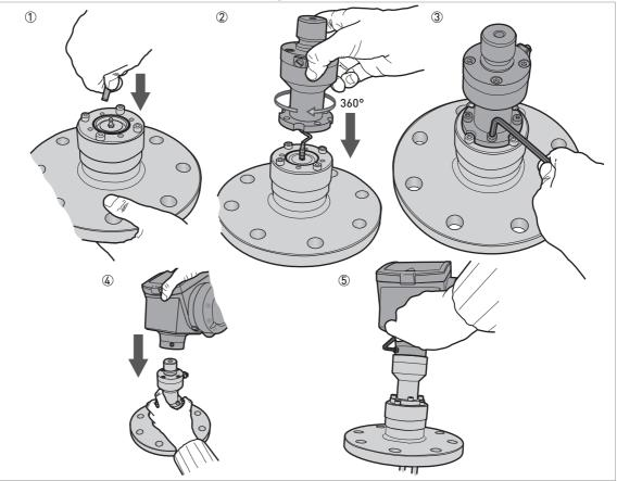
Procedure 3A: How to attach the VF7 signal converter (non-Ex devices)
