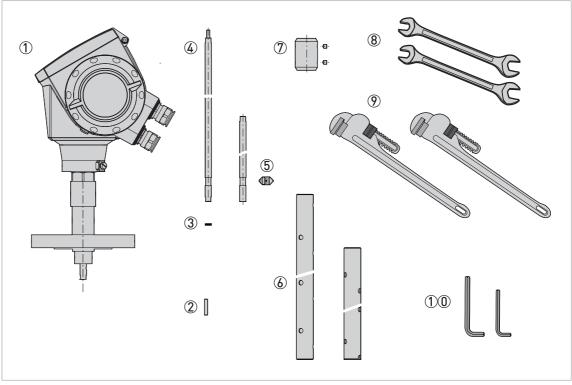
Figure 3-33: Equipment needed to assemble the coaxial probe
