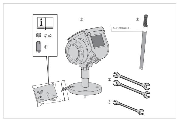
Figure 3-26: Equipment needed to assemble the device
