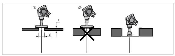
Figure 3-9: Installation on a concrete roof
